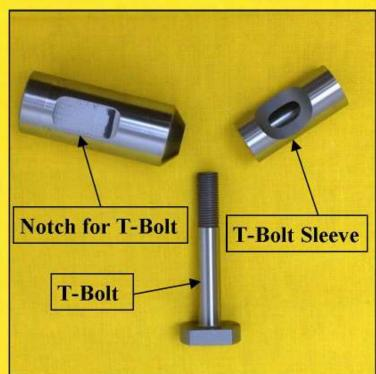
T-Bolt's can be installed on any 1st / Cone / Upset blocks.
